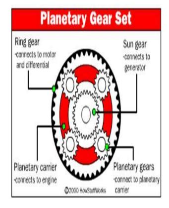
The power split device also allows the car to operate like a series hybrid -- the gasoline engine can operate independently of the vehicle speed, charging the batteries or providing power to the wheels as needed. It also acts as a continuously variable transmission (CVT), eliminating the need for a manual or automatic transmission. Finally, because the power split device allows the generator to start the engine, the car does not need a starter.
