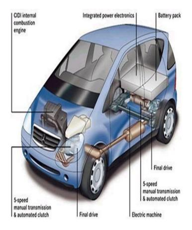
Gasoline engine - The hybrid car has a gasoline engine much like the one you will find on most cars. However, the engine on a hybrid is smaller and uses advanced technologies to reduce emissions and increase efficiency.
